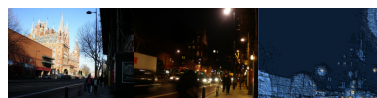
Fig. 3: Images of Saint Pancras Station. From the left to right: day-time image, night-time image and luminance pattern image generated by imagelum software from measurements collected in the field.
