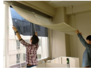
Fig. 4: Setting ND filter
