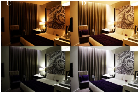
Fig. 3: Picture of the lighting conditions. A. Dim WW; B: Bright WW; C: Dim CW; D: Bright CW
